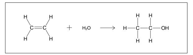
This 'hydrolysis' reaction is carried out in a reaction chamber, at a pressure of 6000-7000 kPa and a temperature of 300  $^{\circ}$ C.
